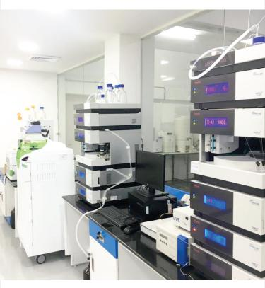
Latest HPLC process to check the % of purity of drugs
